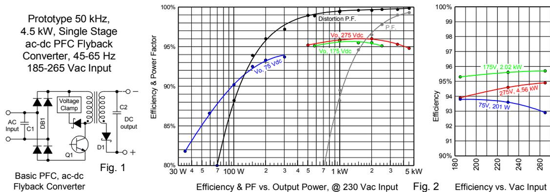
In a PFC flyback the input bypass capacitor C1 needs to be moved to the ac side of the bridge rectifier DB1 (Fig. 1) to prevent distortion of the ac input current. The capacitive input current is  $\approx 10\%$  of full load, resulting in a leading power factor (PF) at lighter loads (Fig. 2), but this is generally beneficial, by compensating in part for the lagging power factor of motors and distribution transformers. And the "distortion PF" from harmonic currents is considerably better.
